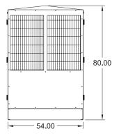
All enclosures are 150 MPH Wind Rated. Level 2 & 3 enclosures include sound attenuation foam.
