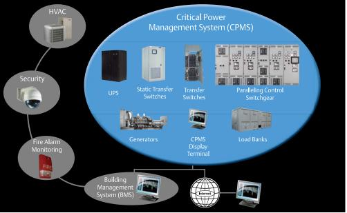
PowerQuest<sup>®</sup> provides monitoring, alarming and control of Critical Power Management Systems, which comprise transfer switches, paralleling control switchgear, gensets, circuit breakers, distribution and other gear. It also integrates with building management systems.
